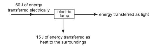
Calculate the percentage of the energy transferred electrically to the lamp which is transferred as light.
