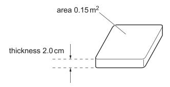
Calculate the weight of the piece of glass.
