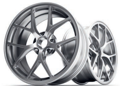
▲ Figure 2.36 Alloy wheel made by 3D printing
