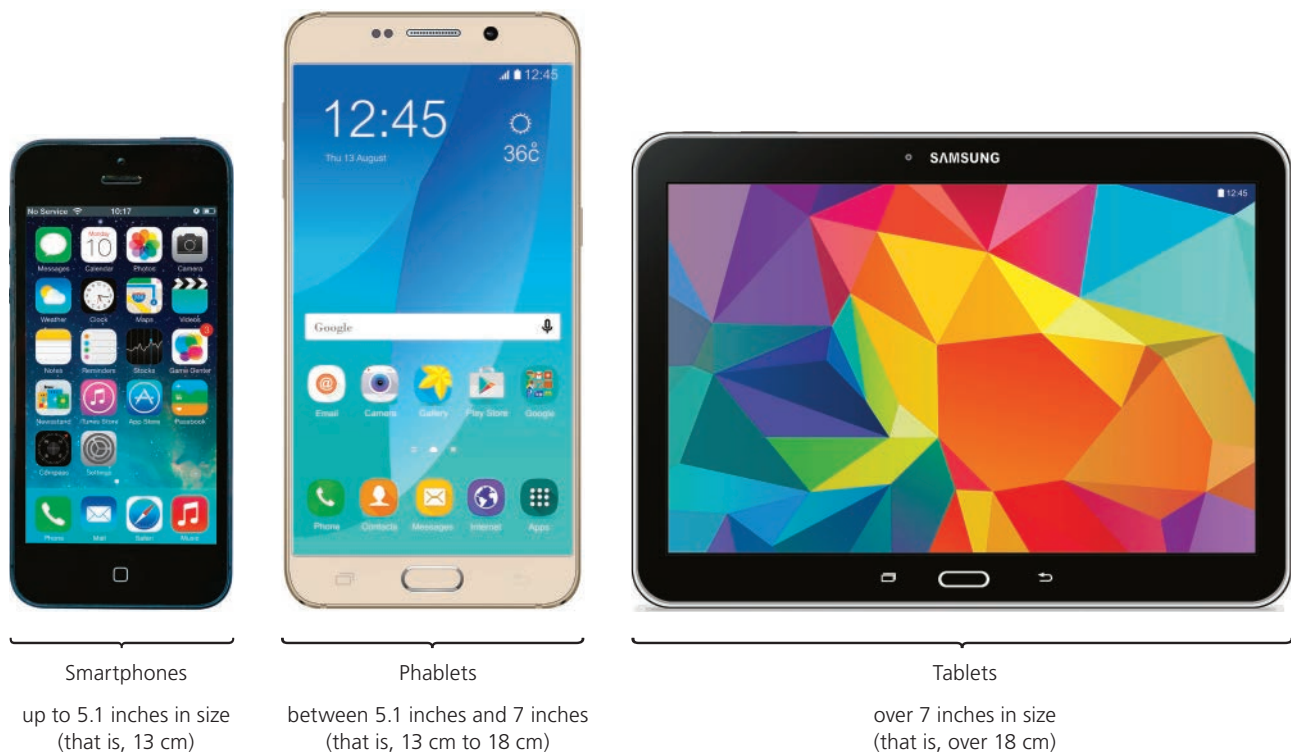
▲ Figure 1.14 Comparison of smartphone, phablet and tablet
