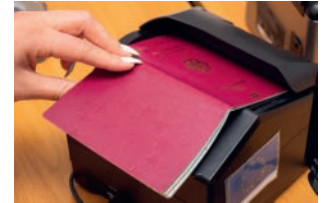
▲ Figure 2.23 Using OCR to process a passport
